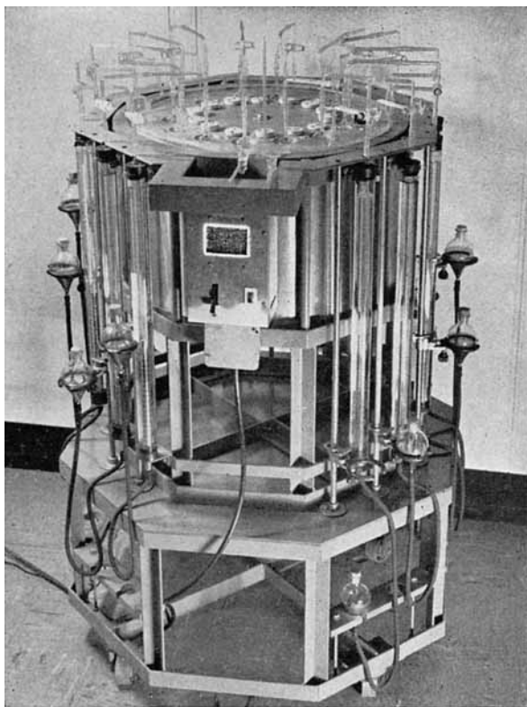
Fig. 1. Front view of volumetric gas-absorption apparatus.
